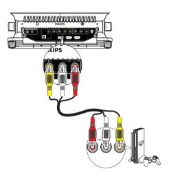
You can also connect the supplied AV switch cable to the AV FRONT jack first, then connect the AV cable to the AV output jacks on the DVD player.
